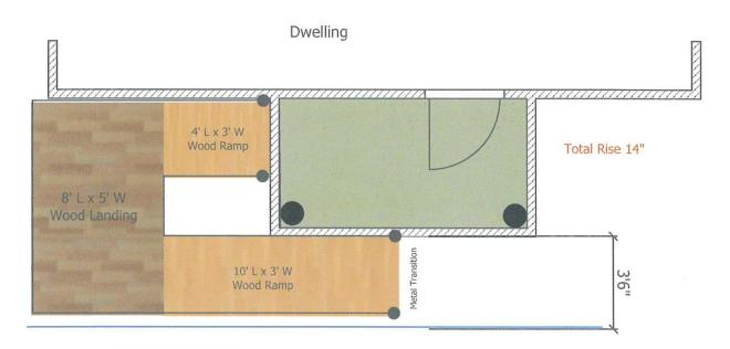
County code does not allow the ramp to be 3'6" past edge of porch. Client has filled out a variance for project.
